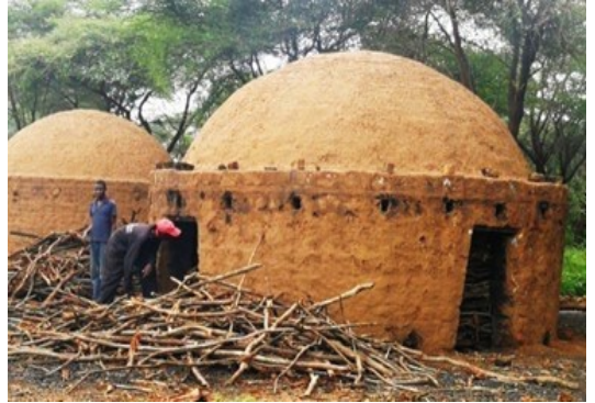
Management of Prosopis by utilization using half-orange kiln for efficient charcoal production in Marigat
