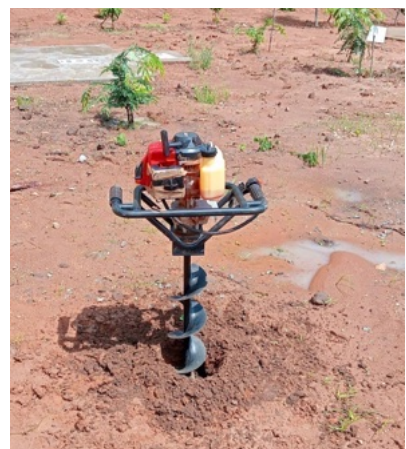
Mechanised hole drilling to break soil hard pan and enhance survival and establishment of seedlings
